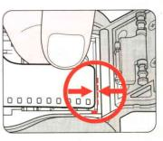
3 Turn on the power switch and load film. Pull the film leader out to the red index
